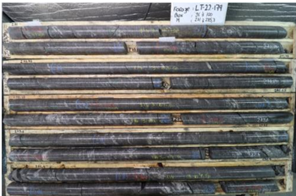
Figure 10.6.3: Photo of paragneiss in hole LT-22-179.
