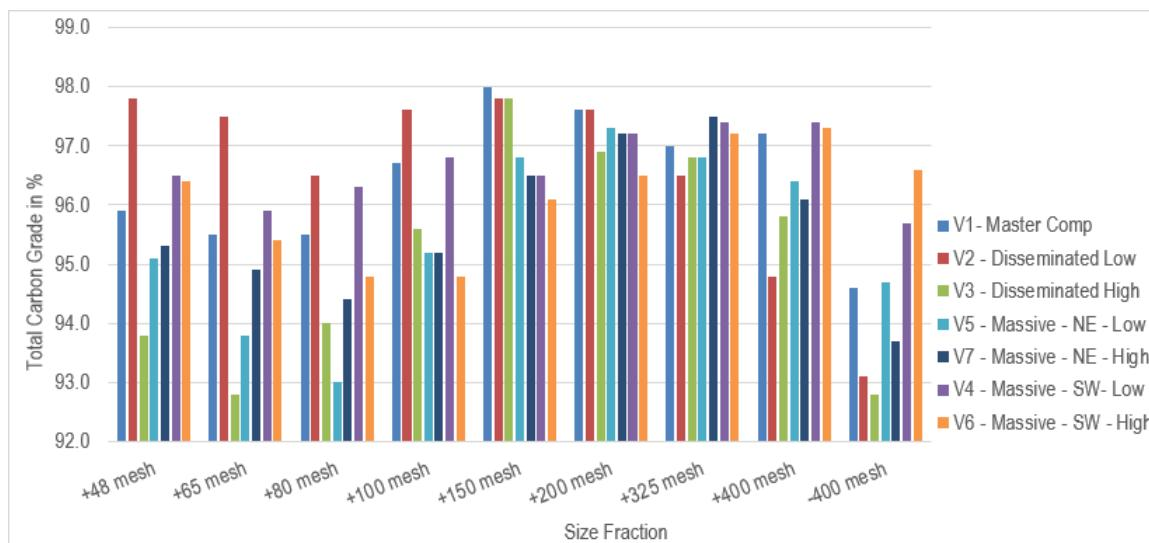
**Figure 13.10 – Variability Flotation Tests (V1-V7) Size Fraction Analysis, Mass Recovery**
